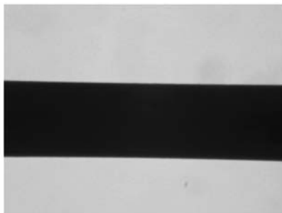
(a) 直线度好的狭缝 (a) Good straightness slit
